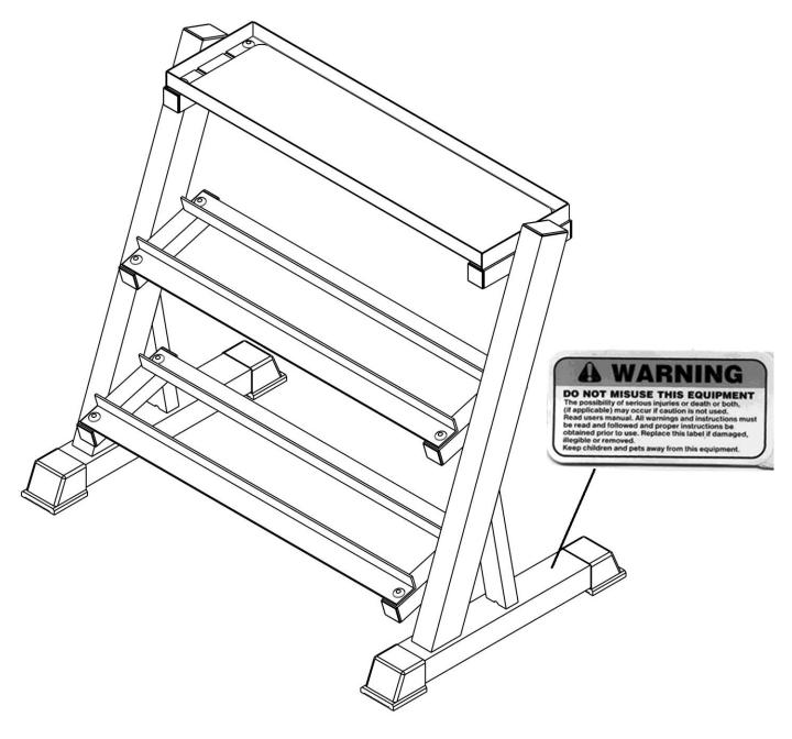
The Warning Label shown here has been placed on the base of Upright Beam. If the label is missing or illegible, please call customer service at 1-800-999-8899 for replacement. Apply the label in location shown.
